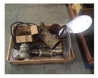
At a Water Reclamation Facility (WRF) in Maryland, a dozen Landia submersible mixers have finally had their motors replaced after nearly 20 years of service – yet the original stainless steel propellers are still intact and set for another lengthy spell in the plant's oxidation ditches.
